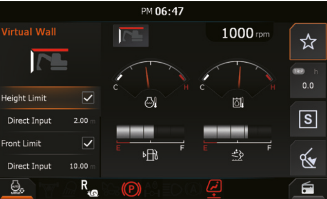
Virtual wall system allows safe operation inside buildings
