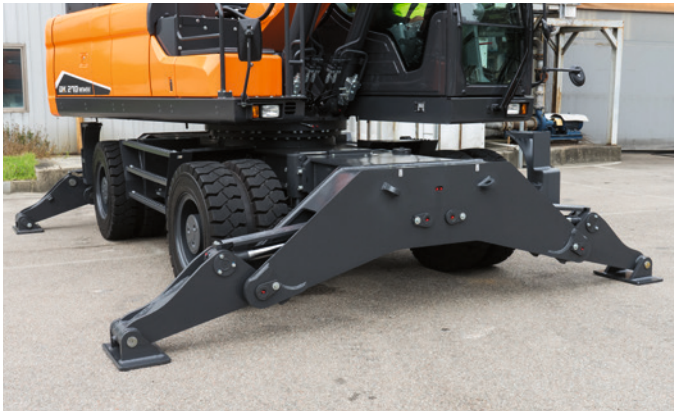
Purpose designed undercarriage with wide outriggers for enhanced stability
